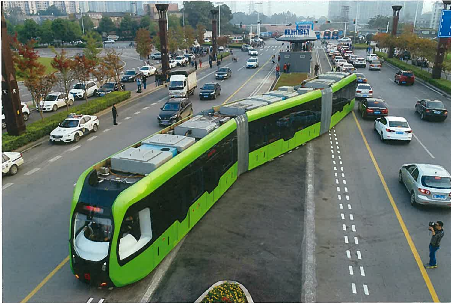
The battery-powered trackless tram, or ART, in operation in Zhuzhou, showing the trackless autonomous guidance system. CRRC Zhuzhou Institute, Author provided
