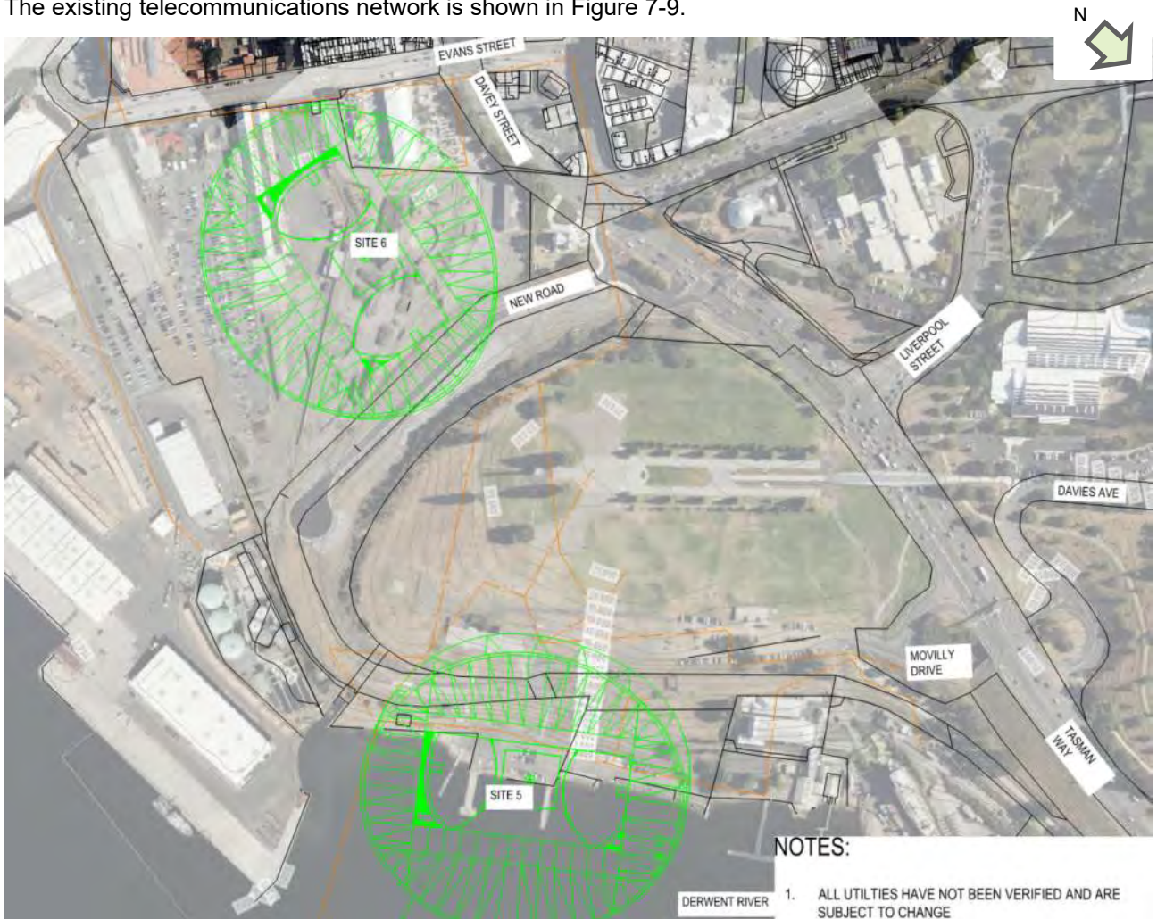
Figure 7-9 – Existing Telecommunications Layout
