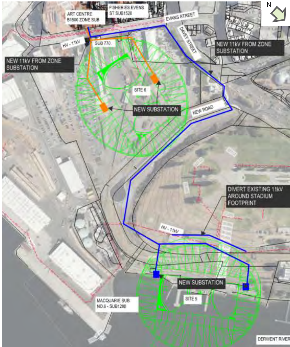
Figure 7-8 - Proposed Electrical Layout
