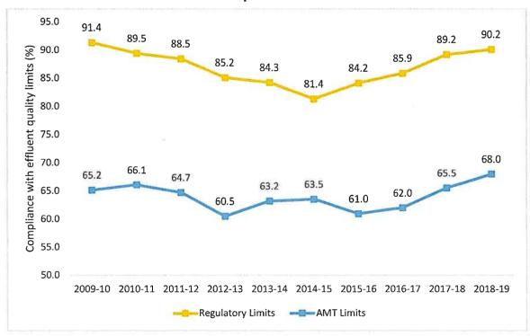
Figure I - L2 WWTP compliance with effluent quality limits for discharge to waters
