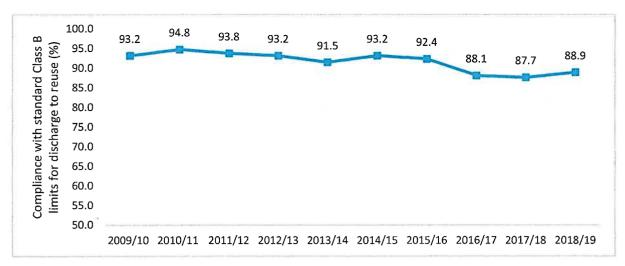
Figure 2 – L2 WWTP compliance with standard Class B limits for discharge to reuse schemes Compliance metrics
