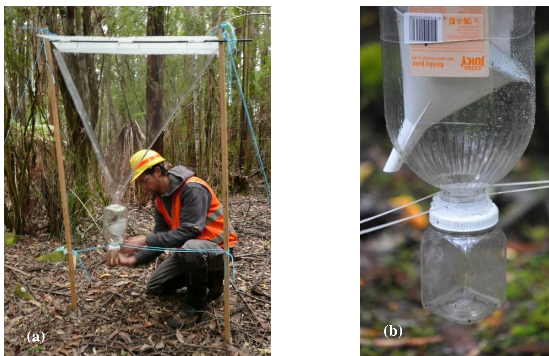
Figure 15. Transparent window intercept trap (a) with a water diverter installed above the collection bottle (b).
