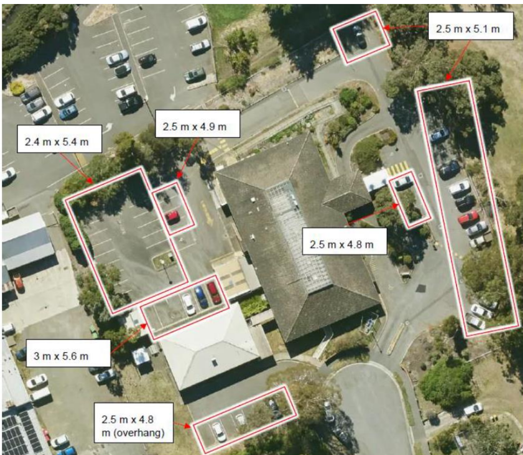
Figure 2 non-compliant parking space across the site, minimum parking bay size is 2.6 m x 5.4 m under AS2890
