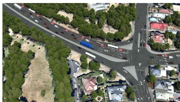
Image 1: Proposed Southern Outlet Transit Lane intersection depicting transit lane approach and realigned intersection, traffic islands and crossings.
