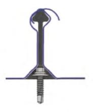
Figure 1.8: FreeForm™ detail of lap before seaming.
