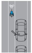
Sandy Bay Road bike lane - constructed 2014-16. Showing risks typical of Hobart's painted bike lanes. The cyclist is exposed to both a 'dooring risk' and minimal space. Many cars do not provide a 1m overtaking gap when overtaking. The speed limit is 50 km/hr.
