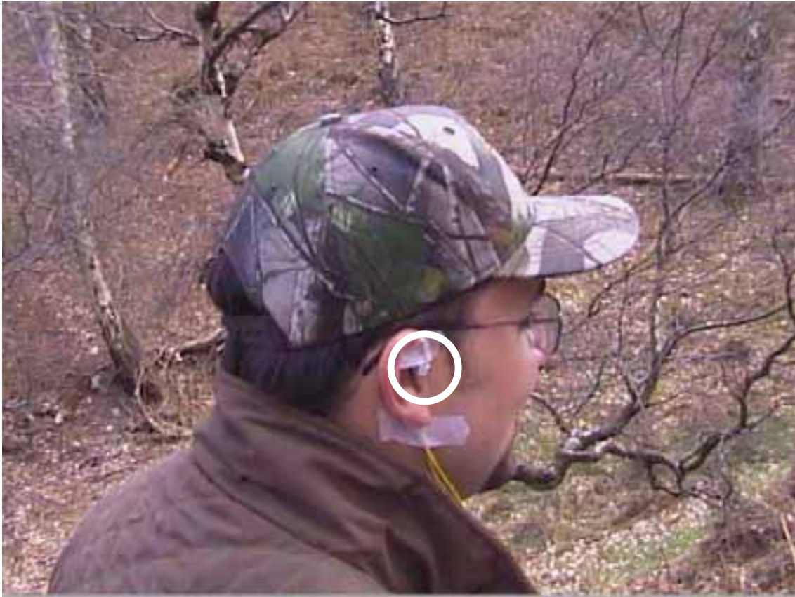
Figure 2 Miniature microphone on the ear for measurements under the muffs
