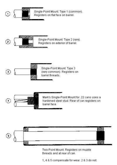
Our testing has indicated that a rifle with a suppressor held in place with a properly executed, two-point, conical, tensioned barrel mount will remain in zero. This zero remains even after the suppressor has been removed for cleaning and replaced. As long as the replacement torque is about the same, the zero will be unaffected. We are talking about no discernable, cold shot shift after a day, week or year, at 180 m or 200 yards.
