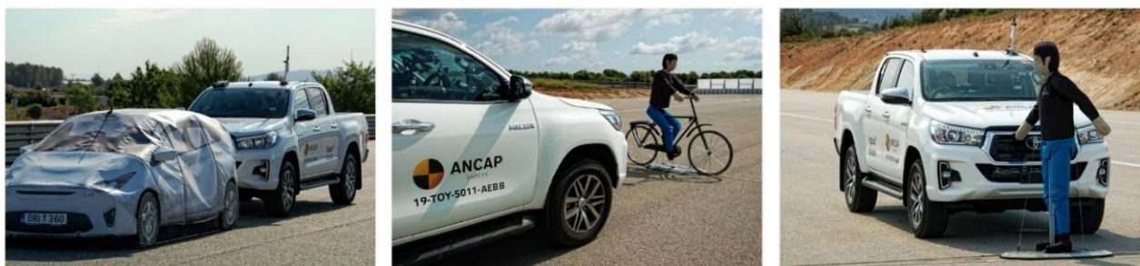
Figure 8 - AEB Scenarios: Car-to-Car rear, Car-to-Cyclist and Car-to-Pedestrian
