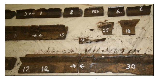
Figure 8. – Broken rusted rail taken from a crossing after the rail causing a derailment
