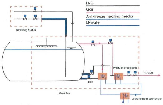
LNGPac Gas Storage System - Suitable for reciprocating engine option.
