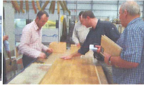
Figure 12: Quality control in flooring system 19mm finished product (350x70) with 3mm surface layer. (Photo P. Volker)
