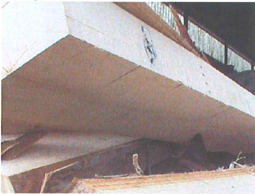
Figure 16: Globulus beam in the green mill, showing little or no defect.
