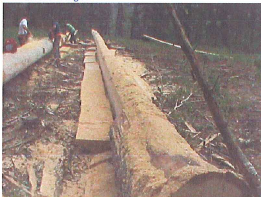
Figure 19: Cutting 30m x 30cm x 30cm globulus beams in the bush using chainsaws for use in mussel barges.
