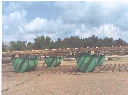
Figure 17: Globulus beams are used to build these 30m x 27m mussel barges.
