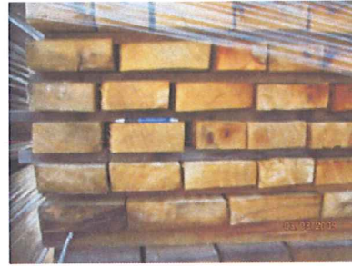
Figure 27: E. globulus boards showing little end checking or collapse. (Photo T. Jaeger)
