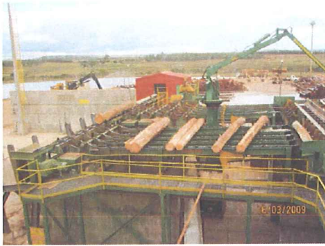
Figure 70: Urofor, log intake deck (Photo T. Jaeger)
