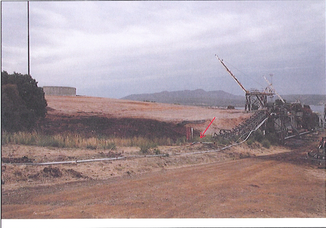
PHOTOGRAPH: 1. Fire origin on Southern end of conveyor belt frame.
