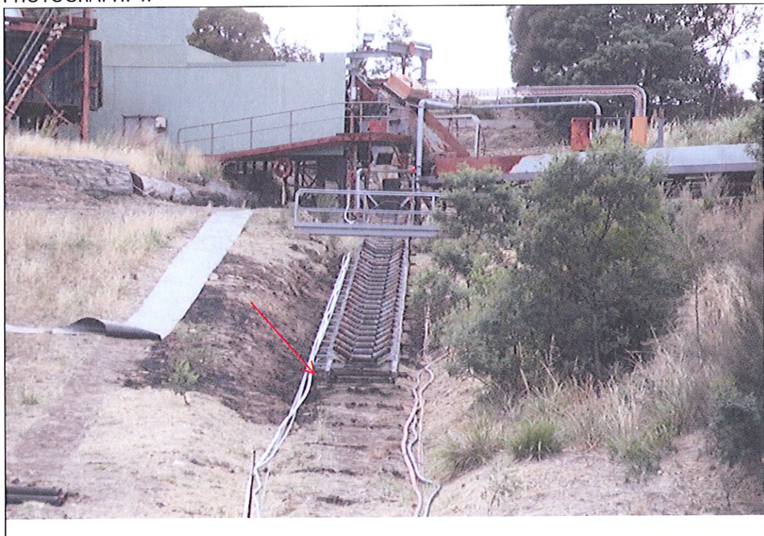
PHOTOGRAPH: 5. Fire origin on northern end of conveyor belt frame.
