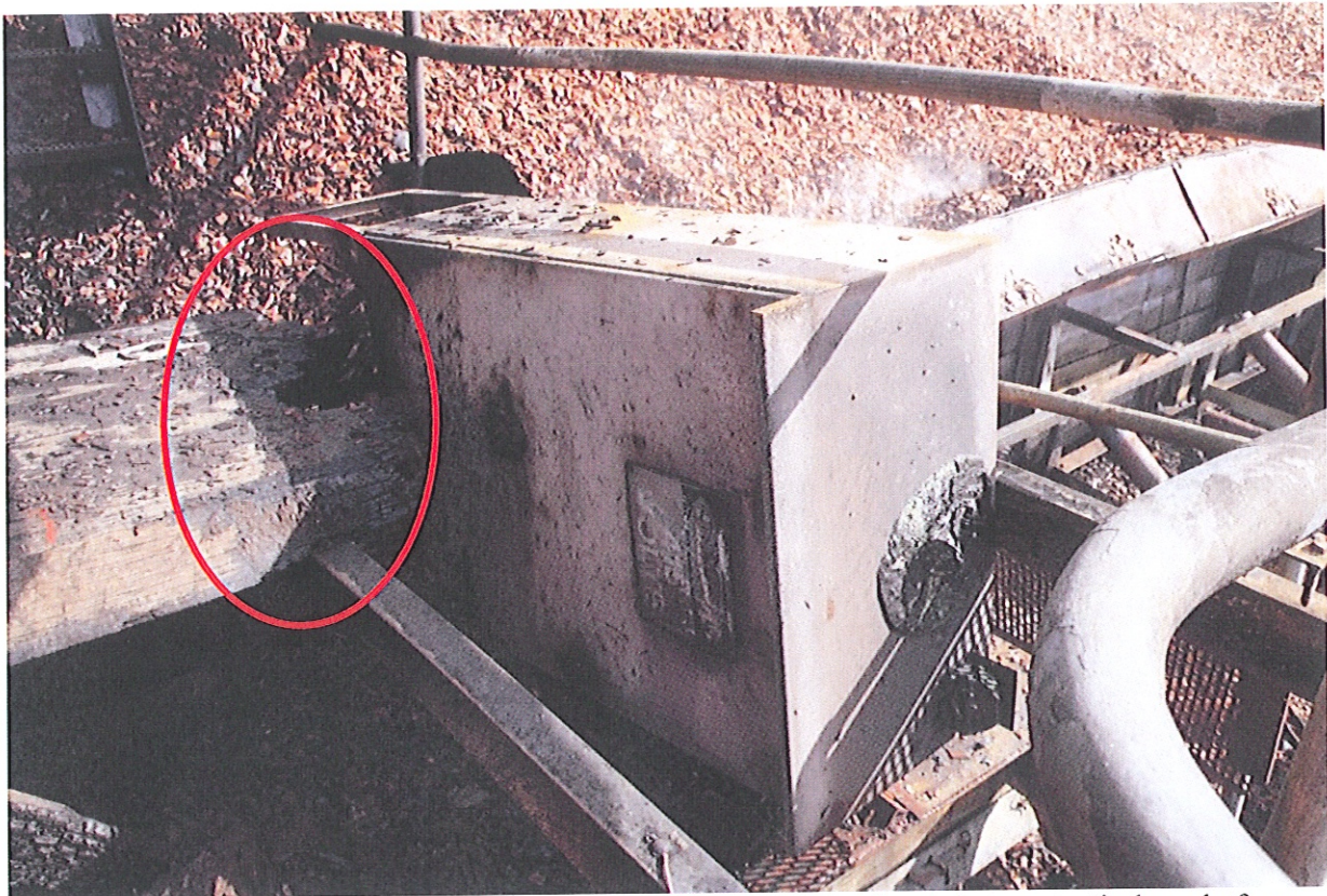
PHOTOGRAPH: 11 Main switch above area of origin. Most overhead damage to timber platform
