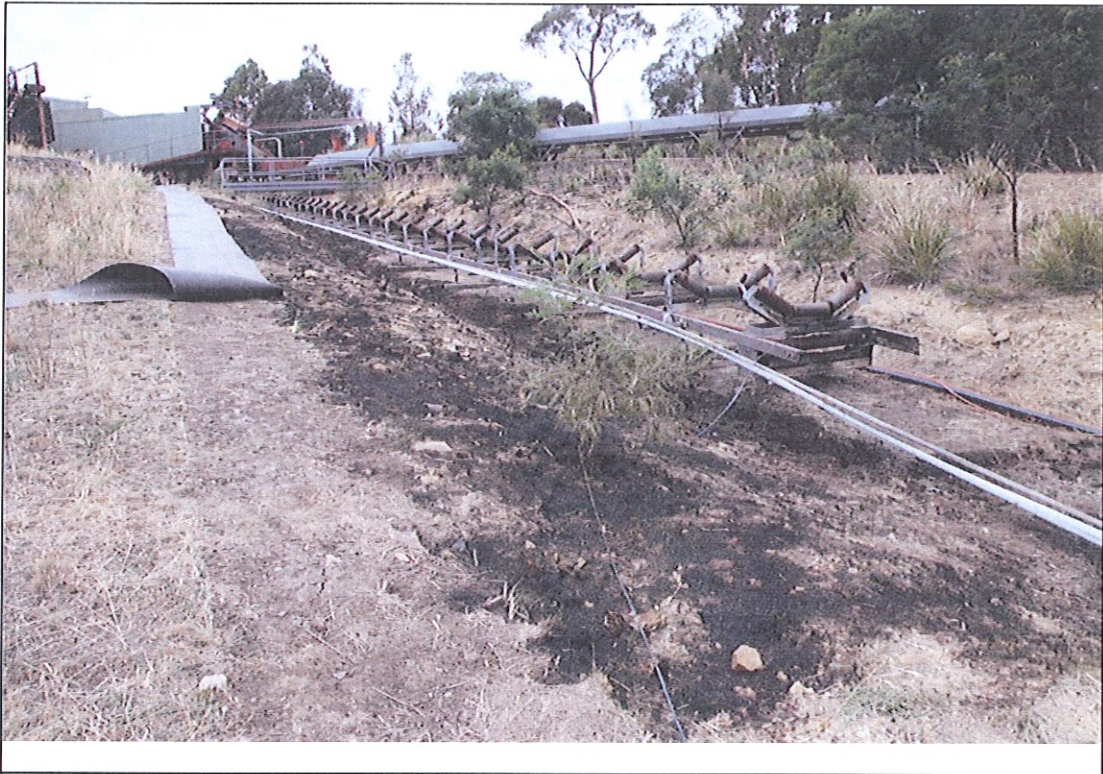
PHOTOGRAPH: 6. Fire origin on northern end of conveyor belt frame.
