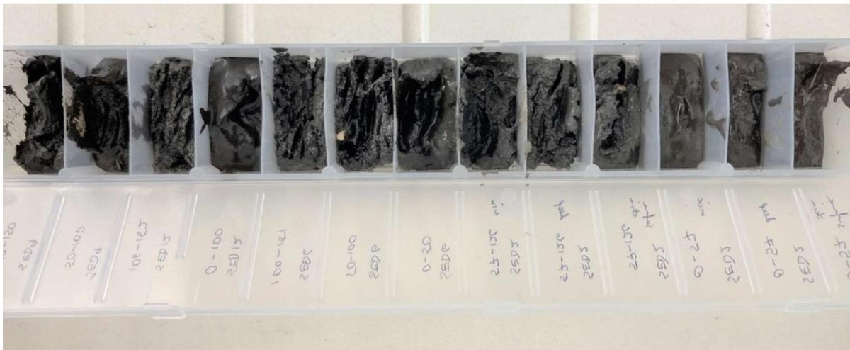
**Figure 101.** Chip-tray incubation of acid sulfate sediment.
