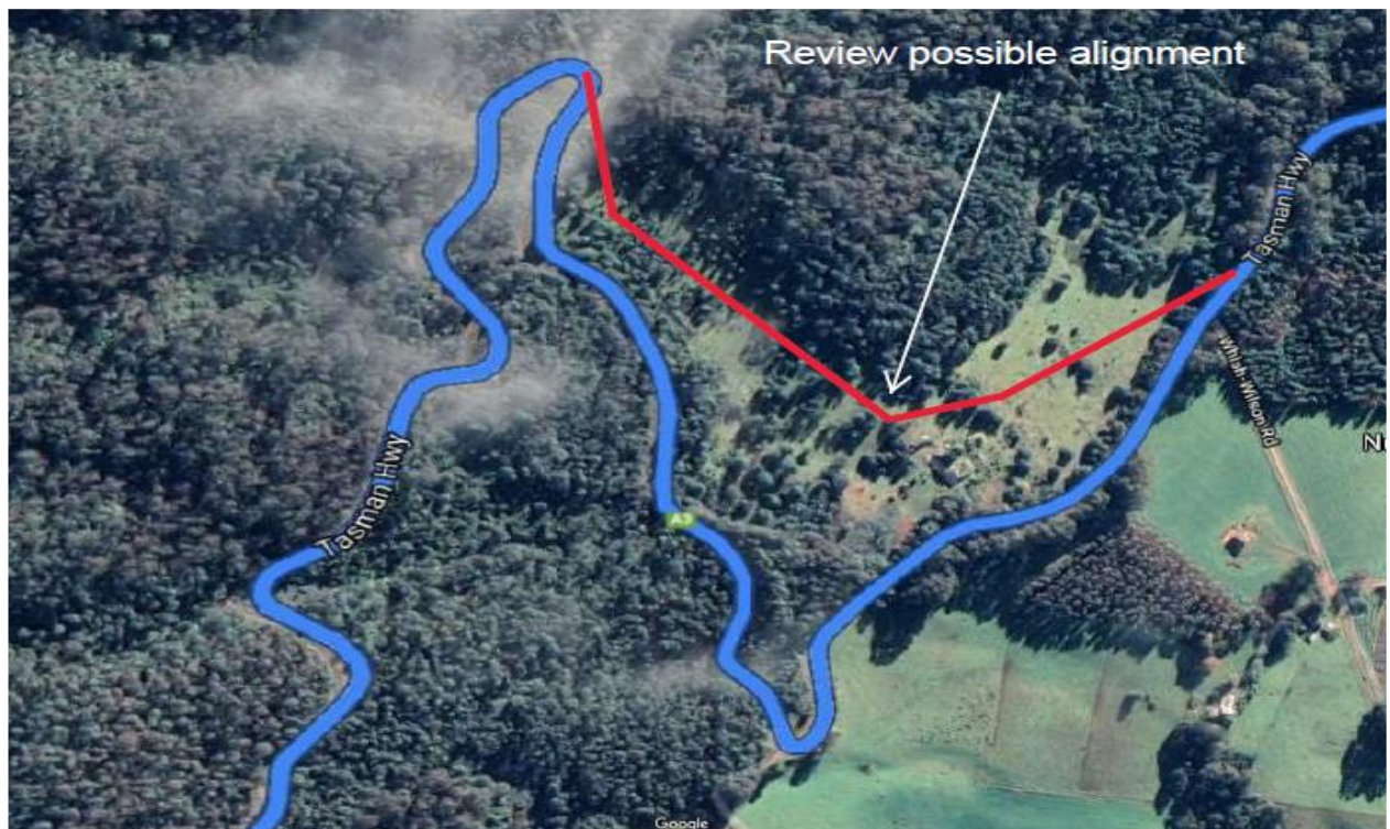
Figure 4: Possible realignment between the Sideling Lookout and Minstone Road discounted due to a vertical grade of 15% over a 700m length of road
