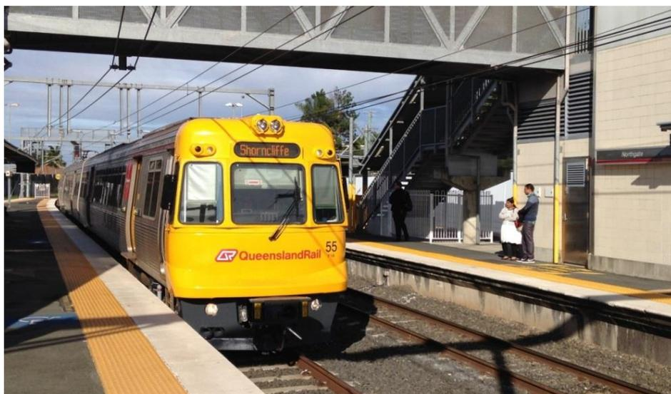
Figure 3: Queensland Rail EMU on narrow gauge (1067 mm)
