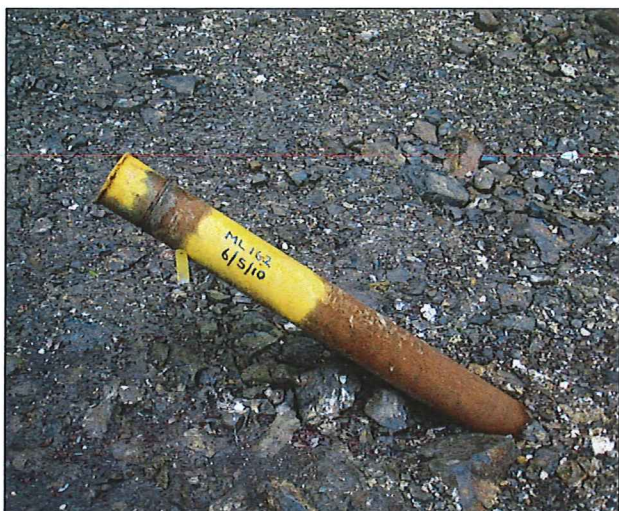
Steel collar — secure, sealed, but number will fade.
