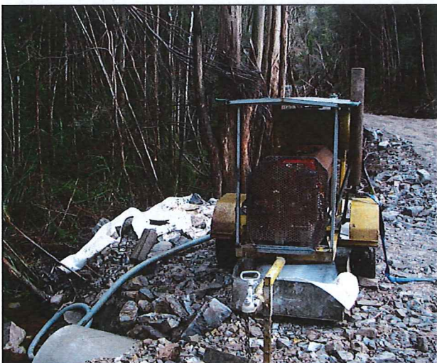
Roofed pump, fuel tank and bund.
