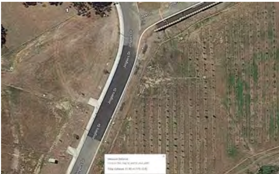
Figure: Google map image showing 50 m section of road and kerb replaced due to subsidence caused by groundwater eroding road base and subbase.
